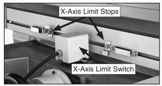
Figure 40. X-axis limit switch and stops.
